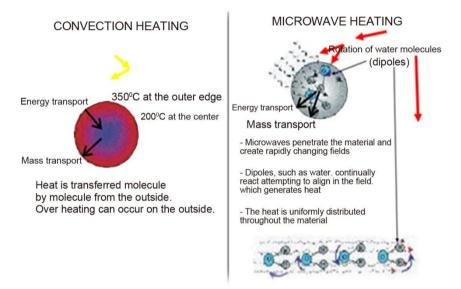
Fig. 1. Energy transfer comparison.
