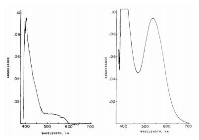
*Figure 6.5* Absorbance spectrum of reagent blank (left) and arsenic (2  $\mu$ g; right) recorded against a SDDC method using spectrophotometer.
