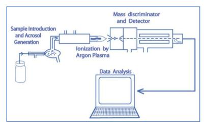
Figure 6.9 Schematic diagram of ICP-MS.
