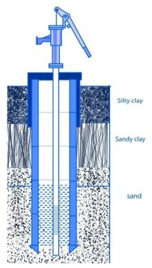
Figure 7.5 Schematic diagram of dug well with sanitary protection.
