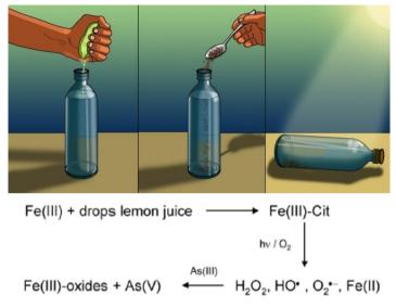
Figure 7.8 Solar-light assisted arsenic removal (Litter et al., 2010).
