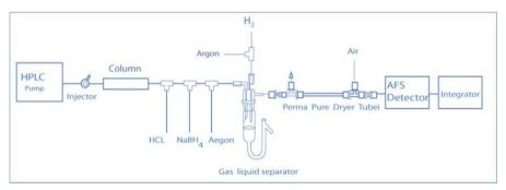
*Figure 6.8* Diagrammatic scheme of HPLC-HG-AFS (PS Analytical application note 024).
