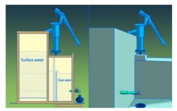
Figure 7.2 Schematic diagram of pond sand filter.
