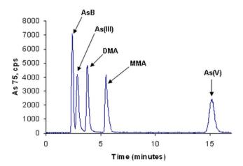
*Figure 6.10* Typical HPLC-ICP-MS chromatogram of an arsenic multianalyte working standard solution (5 ng/g).
