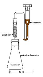
Figure 6.4 Schematic diagram of arsine generator.
