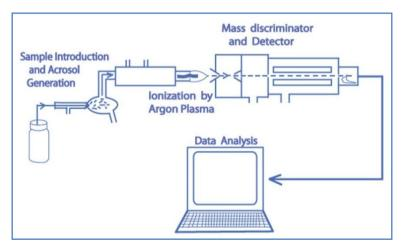
Figure 6.9 Schematic diagram of ICP-MS.
