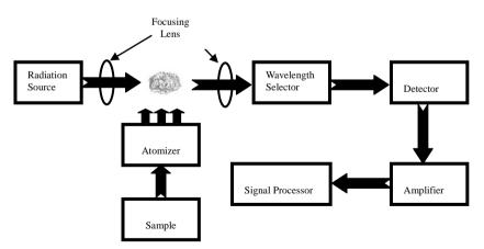
Figure 6.6 Schematic diagram of atomic absorption spectrometer.
