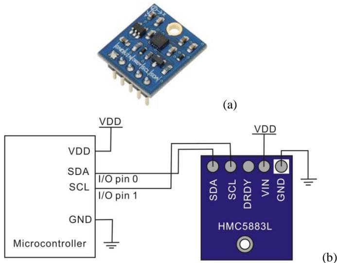
**Figure 3.10** Compass module (a) and the schematic (b).
