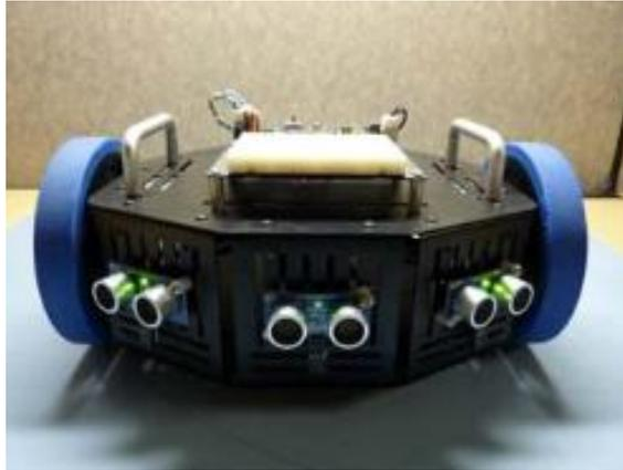
*Figure 3.9 Avoider robot using 3 PING))) on the body.*
