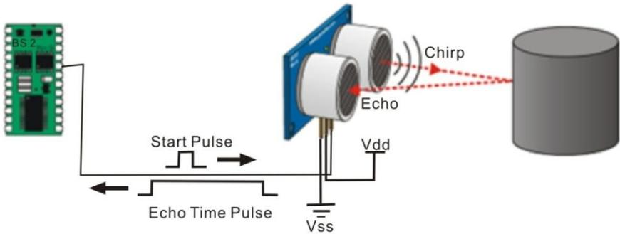
**Figure 3.6** The basic principle of ultrasonic distance sensor [2].
