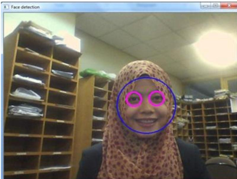
**Figure 9.2** Result of face detection using Haar classifier.
