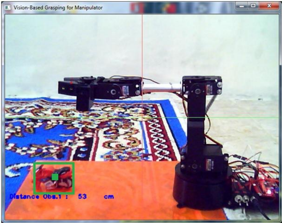
Figure 12.7 Object detection and grasping OpenCV.
