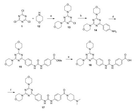
Scheme 4. Reagents and conditions. (a) Et<sub>3</sub>N (5q.), acetone, crushed ice, -20 ℃-0 ℃;
