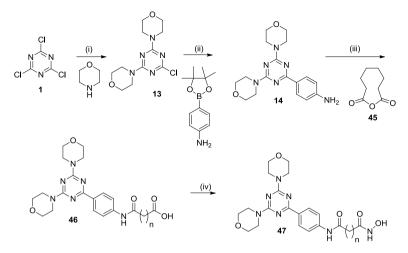
Scheme 12. Reagents and conditions: (i)  $Et_3N$ ,  $CH_3COCH_3$ ; (ii)  $Pd(Ph_3)_4$ ,  $K_2CO_3$ , DMF; (iii) THF, 0  $^{\circ}C$ ; (iv)  $NH_2OH.HCl$ , ClCOOBu-i, THF.
