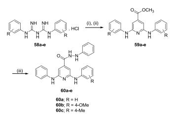
Scheme 15. Reagents and conditions: (i) NaOCH<sub>3</sub>, CH<sub>3</sub>OH, room temp 3 h; (ii) dimethyloxalate, CH<sub>3</sub>OH, NaOCH<sub>3</sub> reflux, 12 h; (iii) phenylhydrazine, EtOH, AcOH, reflux 18 h.
