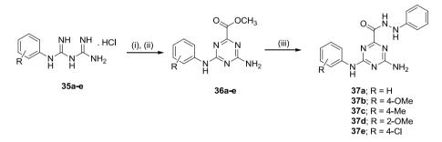
Scheme 9. Synthesis of 4-amino-6-(arylamino)-N-phenyl-1,3,5-triazine -2-carbohydrazides (3a-e). Reagents and conditions: (i) NaOCH<sub>3</sub>, CH<sub>3</sub>OH, rt, 3 h; (ii) dimethyloxalate, CH<sub>3</sub>OH, reflux, 4 h; (iii) phenylhydrazine, AcOH, EtOH, reflux, 12 h.
